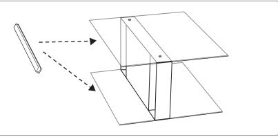
Attach clear rubber floor protectors (Part G) to bottom the fireplace glass and turn it upright. If rubber is longer than the glass, you can cut this to length with a scissor. This is to help protect the glass when standing.
